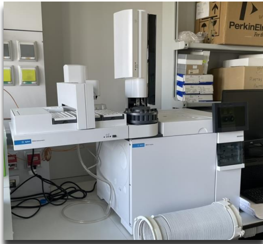
Phospholipid fatty acid (PLFA) analysis using gas chromatography (GC).
